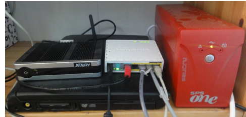
Figure 3. Indoor hardware of a community network node with router, server and cloud resource
