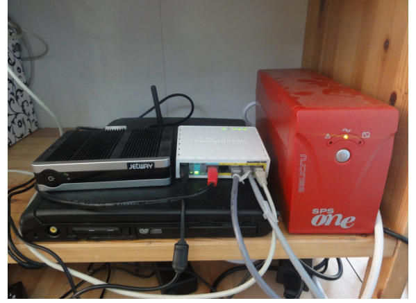
Fig. 3. Cloud resource at a community network node
